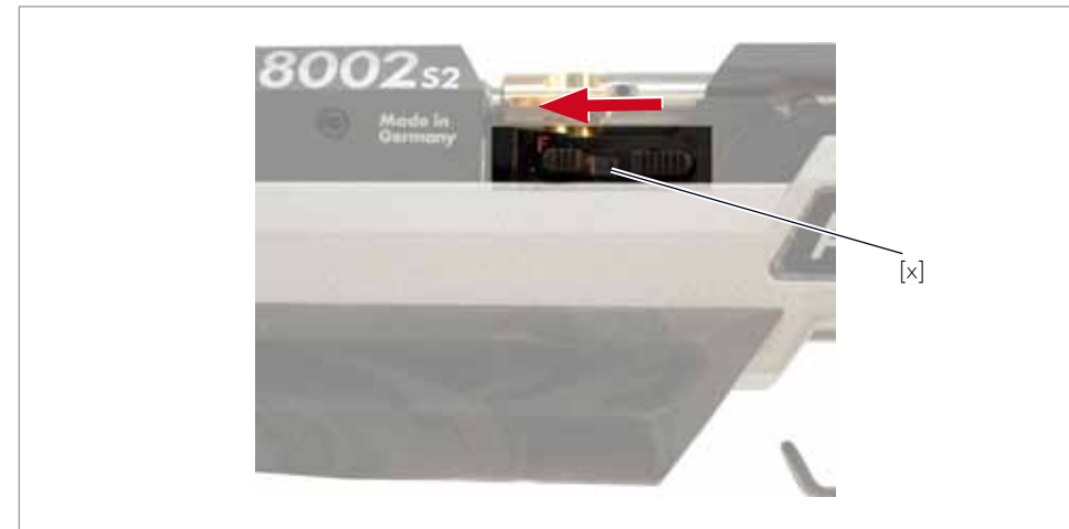
Fig.7 Safety catch "Ready to Fire"
