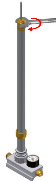
A4. Slide end cap back over tube and re-assemble
