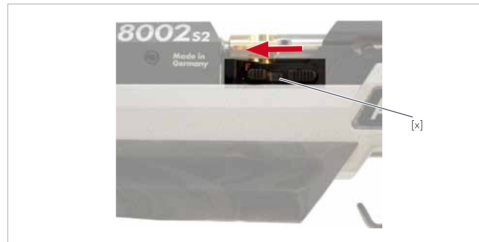
Fig.7 Safety catch "Ready to Fire"
