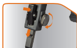
Bipod Legs with 5 Notches (0.68" Apart) for Most Positive Extension, Plus Flexible In-Between Notch Extension; Lock with Wheel and Retract by Press Button
